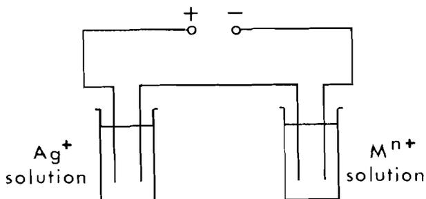
The metals Ag and 'M' are deposited by electrolysis
